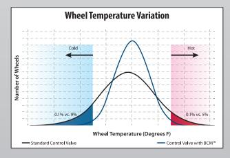
**BCM is good for your bottom line.** There are several ways the Brake Cylinder Maintaining feature of the DB-60 II can reduce your freight cars' lifecycle costs. You'll see more uniform wheel, brake shoe, and rail wear. You'll benefit from lower in-train forces and reduced coupler and draft gear loads. And that means fewer broken knuckles and drawbars that can lead to delays, damage, or derailments.
