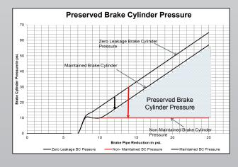
**E<sub>2</sub>O:** restores up to 85% of lost brake force
