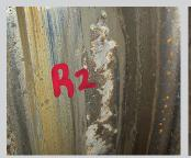
BEFORE: Large surface defects like the one shown on the R2 wheel increase kip forces, causing track and wheel damage.
