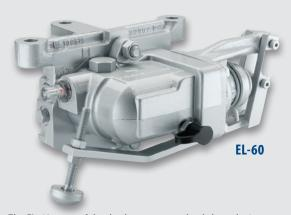
The EL-60 empty & load valve protects wheels by reducing braking forces on empty cars. Available with proportioning levels of 40, 50 or 60%, EL-60 is a fully proportioned, body-mounted design that senses loaded or empty conditions to safely adjust braking power, and features a visual indicator showing full or proportional brake condition.
