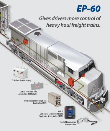
The EP-60 electronically controlled pneumatic brake (ECP) system dramatically reduces in-train forces and benefits you in three important ways.
