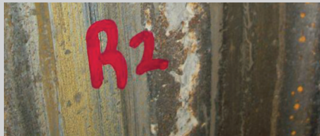
BEFORE: Large surface defect like the one shown on the R2 wheel increases kip-forces, causing track and wheel damage.
