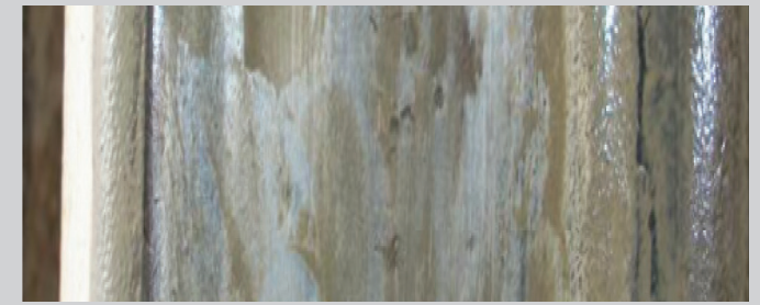
AFTER: During 55 days in service, WheelSaver repaired the tread defect on the R2 wheel.
