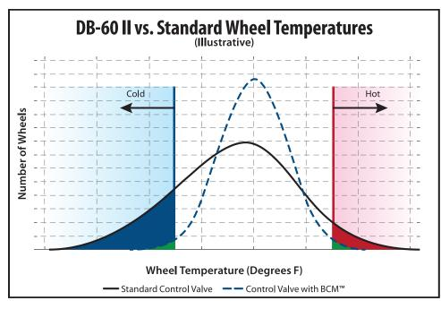
BCM reduces the number of cars with wheel temperatures outside the acceptable limits. On cars with brake cylinder leaks, wheels stay warm while cars without leaks don't have to work as hard and wheels don't get as hot. The result is a more efficient system with far less stress.
