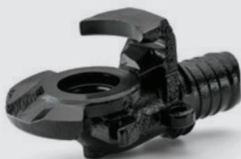
NYAB's LOC-PAD gladhand is engineered to achieve a significant reduction in undesired hose separations. Featuring uniquely placed and raised metal pads that gently 'lock' your hose connection – without undue compression of gaskets – LOC-PAD gladhands reduce lost productivity and wasted fuel caused by unintended hose separations.
