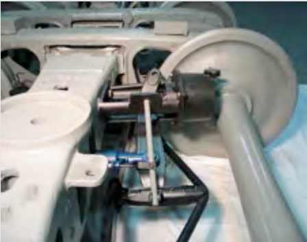
The cylinder-bolster connection is easily-accessible and visible to ensure ease of maintenance.
