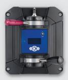
**EBVe** — Our enhanced Electronic Brake Valve (EBV), available in desktop and bulkhead configurations, has fewer parts, non-contacting handle sensors and an IP55 rating that delivers improved reliability as well as a 20-year service life. The unit also includes an ER reduction button with auto bail, allowing the operator to reduce brake pipe pressure 1 psi at a time.
